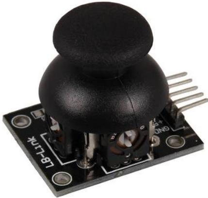
To use the joystick, you also need the ADC. The pin assignment can be found in the table below.
